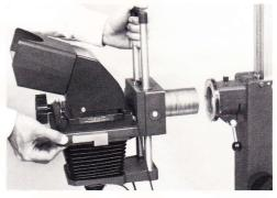
**2.** Attach the camera mount to the vertical carriage in the orientation shown; lock it in place in the same way as the MP-4 camera (tighten retainer screw, then locking knob).
