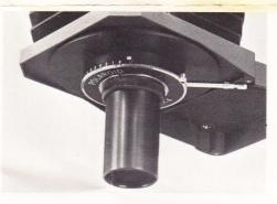
2. Adjust the bellows so that the distance from the film plane to the shutter panel is about 10 inches (25.4cm). This position on the focusing column scale (A) is approximately 22.5 cm. At this distance, the magnification of the picture will be about the same as that indicated by the microscope objective and eyepiece being used.
