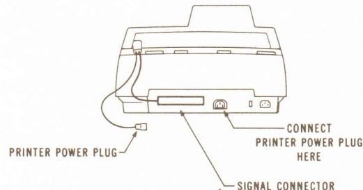
If the rear of the calculator has a receptacle which will accept the printer's power plug, connect the two. If the rear of the calculator does not have the receptacle connect the supplied adapter between the printer's power plug and a wall receptacle.
