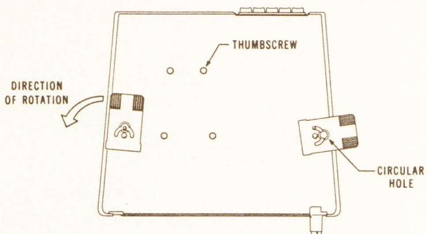
Turn the plastic wings from their stored position to the fully extended position. Notice the two circular holes that have appeared near the pivot point of the wings; they will fit over the thumbscrews on the calculator.
